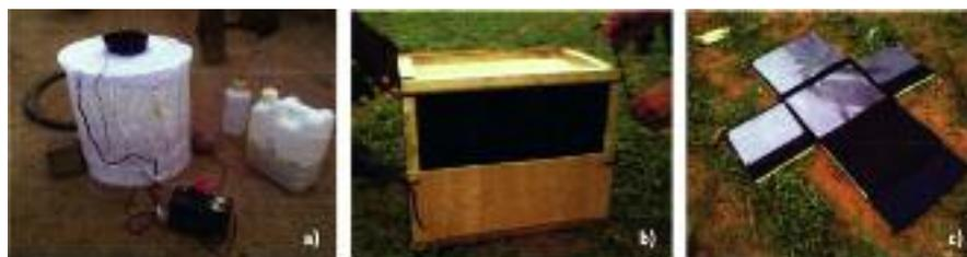
**Fig. 1:** a) BG-Sentinel trap, triggered with BG-lure (not visible) and CO<sub>2</sub> obtained through yeast fermentation (container on the right); b) Sticky Resting Box closed, triggered with a source of moisture (not visible) and ready to be used in the field and c) Sticky Resting Box open, where you notice the internal adhesive surfaces that act as capture systems.
